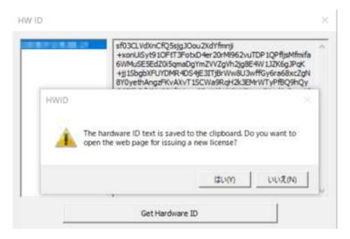
Hwid.exe detects MAC addresses and other hardware properties to calculate a hash from them. It is this hash that is fed to generate the hardware ID. The hash is irreversible to the original data; it cannot be manipulated/exploited to identify your hardware
