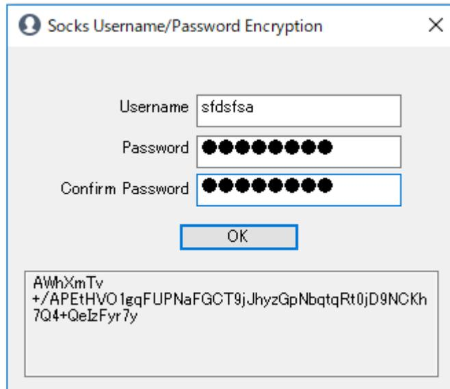
Enter SOCK5 proxy server username and password and press [OK]. The encrypted string will be shown in the lower box. Copy the string and set it to “userpass” key.
