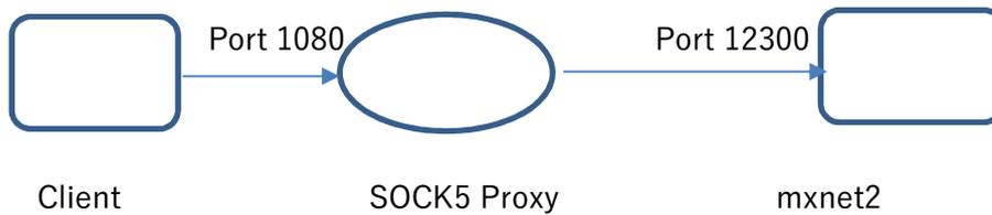
In the client configuration file, create a new section [SOCKSSERVER]. Under the section, specify the IP and port of the proxy server.
